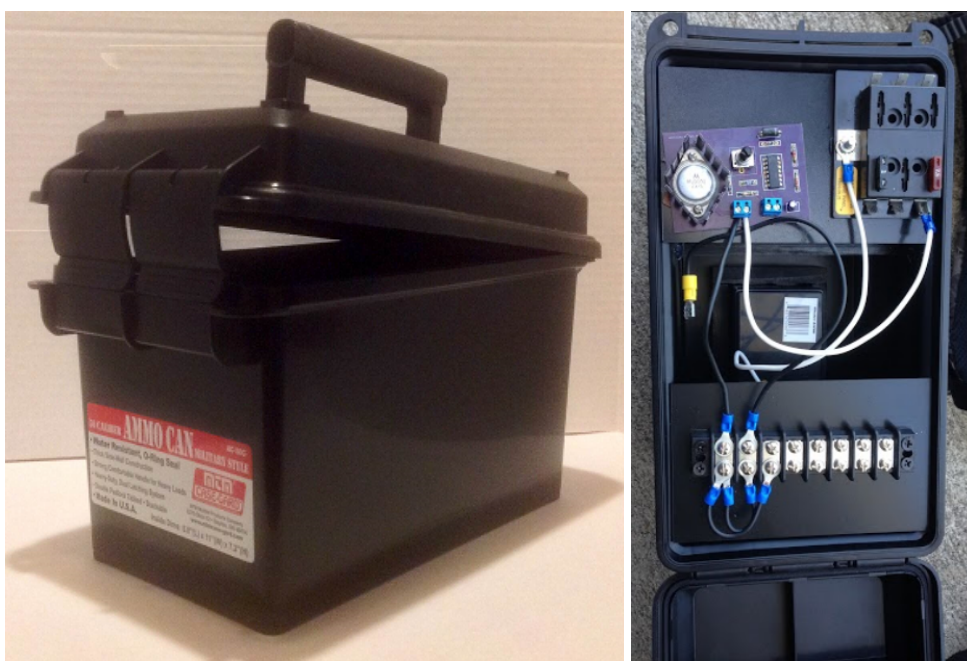
Figure 15 – Power System Housing
