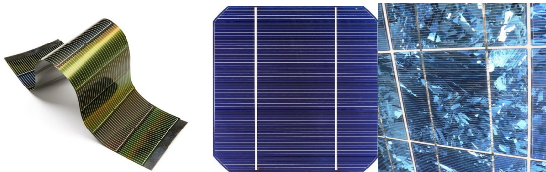
Figure 3 – From left to right a thin-film cell that has been deposited on a flexible plastic substrate a monocrystalline solar cell and a polycrystalline cell. (Permission Requested)
