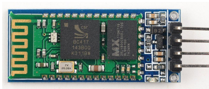
Figure 4.5 - HC-05 Wireless Bluetooth Transceiver Module (purchased/ tested)
