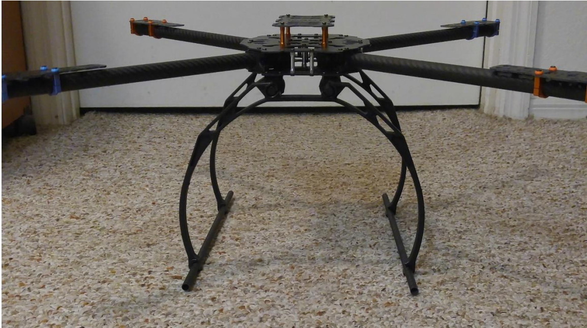
Figure 6.1.1A Tarot Iran Man 650 Frame Assembly
