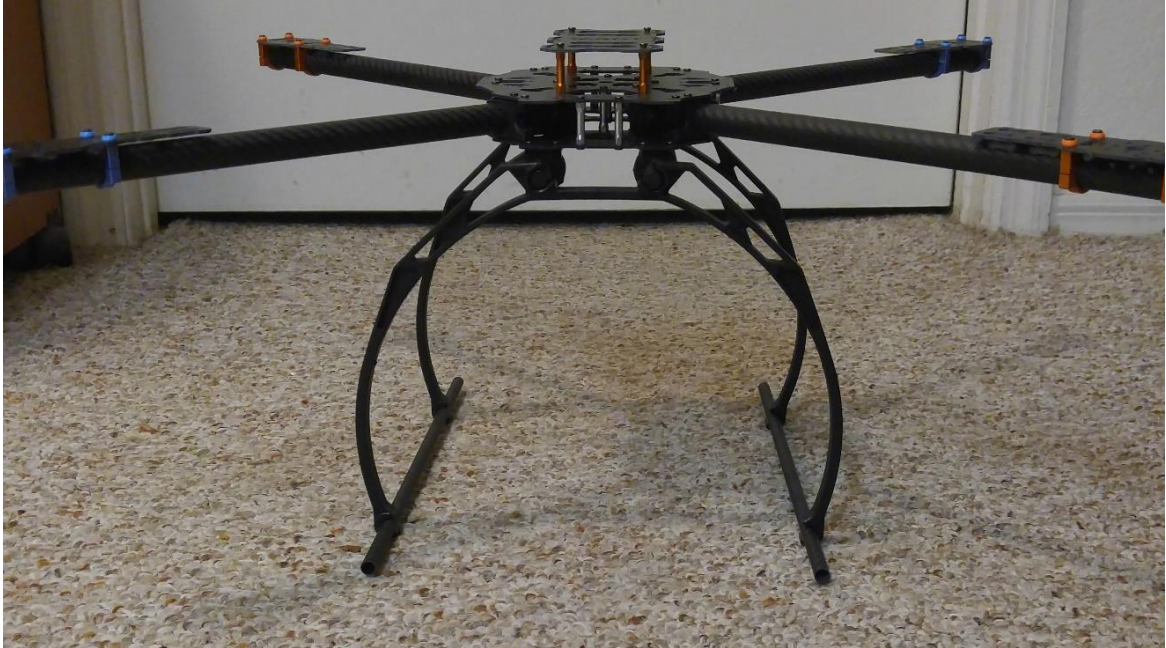
Figure 6.1.1A Tarot Iran Man 650 Frame Assembly
