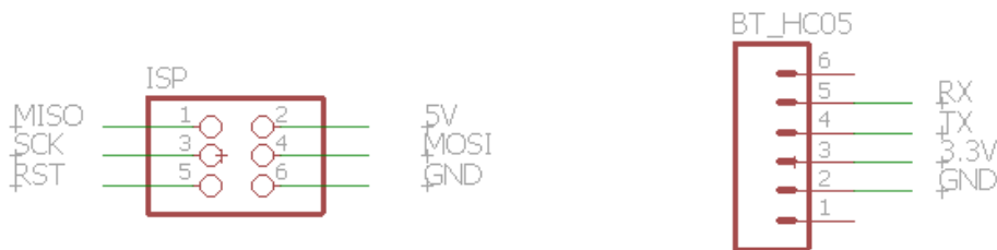
Figure 28: Original Eagle schematic of standard 2x3 ISP configuration and the needed pins for the HC-05. (39)
