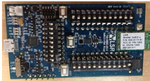
Figure 29: SaBLE-x Development Board
