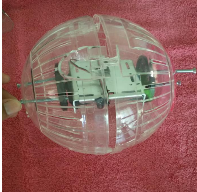
Figure 8-2: Chassis first attached to inside of hamster ball
