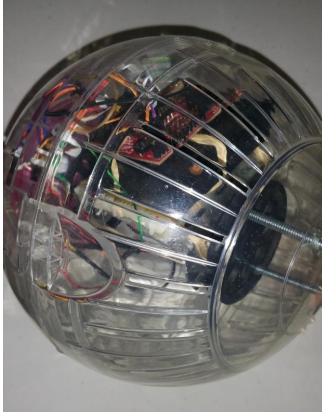
Figure 8-3 Prototype with electronics strapped to chassis
