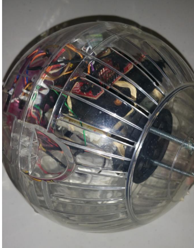
Figure 8-3 Prototype with electronics strapped to chassis
