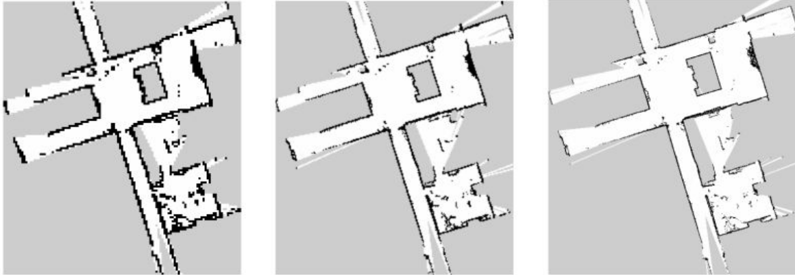
Figure 3.3.3 Examples of HectorSLAM Intermediate and Final Map Outputs (Reprinted with Permission from Stefan Kohlbrecher)
