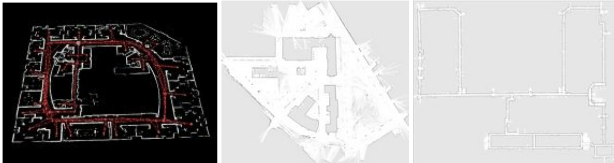
Figure 3.3.2: Examples of GMapping Final Map Outputs (Reprinted with Permission from Cyril Stachniss and Wolfram Burgard)
