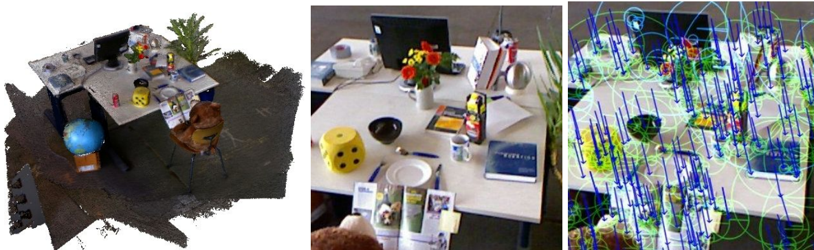
Figure 3.3.1: RGBDSLAM 3D Scan Output (Left), Camera Image (Center), Camera Image with Keypoints Visible (Right) (Permission Pending)
