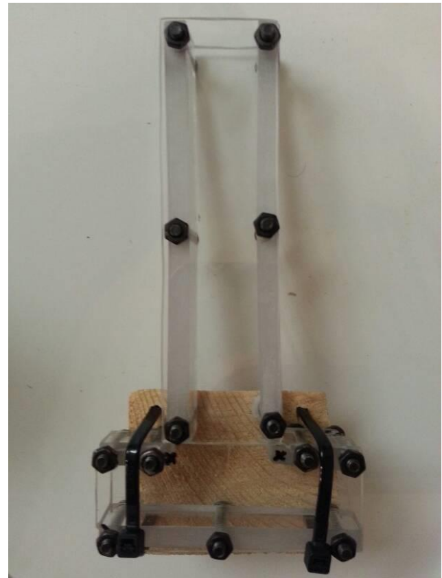
Fig. 5. Fixed magazine holds up to nine projectiles.
