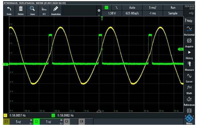
Fig. 11. Oscilloscope input of 12vAC line (yellow) and output of Frequency circuit (green)
