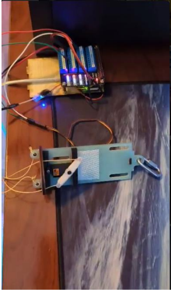
Figure 26: The servo being controlled directly by the Raspberry Pi
