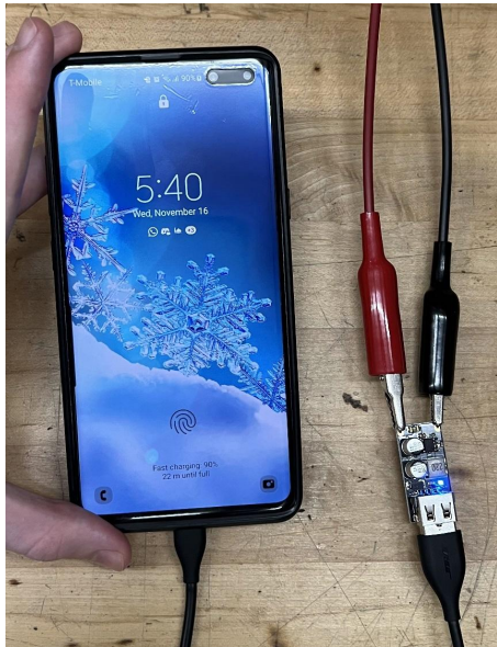
Figure 35: Demonstration of quick charging using QC board
