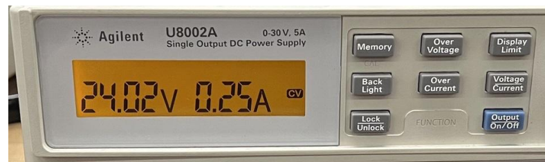
Figure 36: Charging voltage applied to module and current draw
