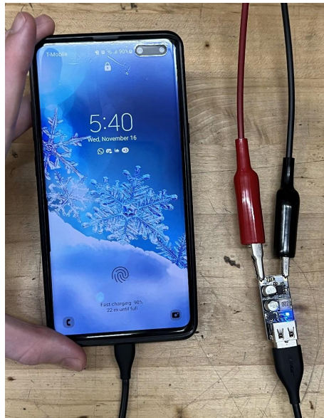
Figure 31: Demonstration of quick charging using QC board
