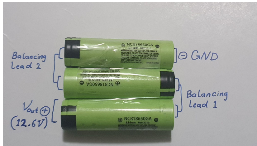
Figure 15: Battery pack configuration of 3 cells on series (3S)
