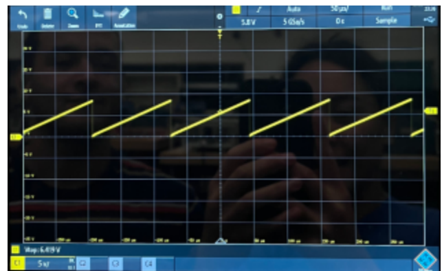
Figure 7.1 Sawtooth Waveform from Testing IC
