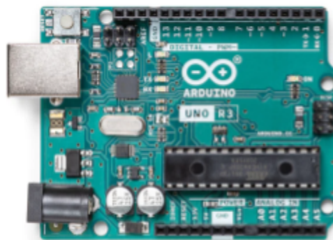
Figure 3.13: Arduino Uno Rev3/ATmega328P
