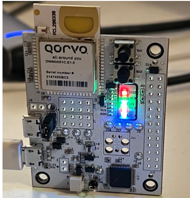
Figure 5-10: Personal Photo of DWM3001CDK Successful Flash
