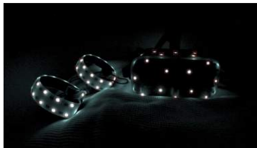
Figure 3.4: Meta Quest 2 infrared tracking system. Reproduction permission requested from Mechatech.
