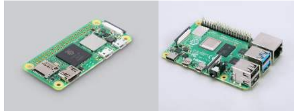
Figure 3.14: Raspberry Pi Zero 2 W (left) and Raspberry Pi 4 Model B (right). Reproduction permission requested from Raspberry Pi.
