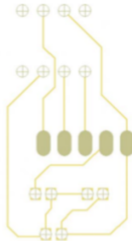
Fig. 53. Drill holes added.
