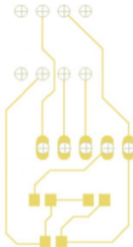
Fig. 58. Drill holes added to 5-pin header.
