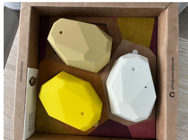
Fig. 4. UWB beacons from Estimote used in the user localization system.
