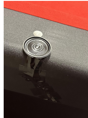
Fig. 3. Speaker used for the user guidance system mounted to the billiards table.
