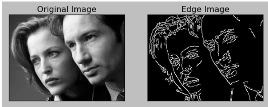
Figure 3.6: Canny Edge Detection on an Image (Awaiting Permission from BogoToBogo)
