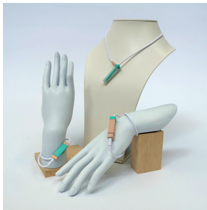
Figure 3.17: Maptic Haptic Feedback Apparatus (“Maptic is a wearable navigation system for visually impaired people”)
