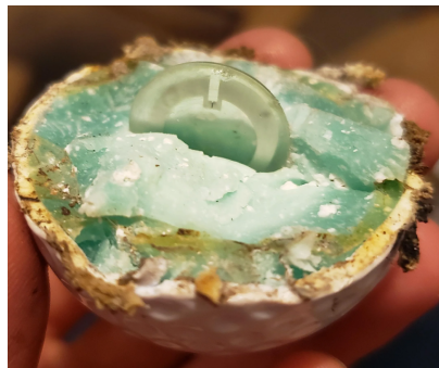
Figure 3.21 RFID Tag Embedded in Golf Ball
