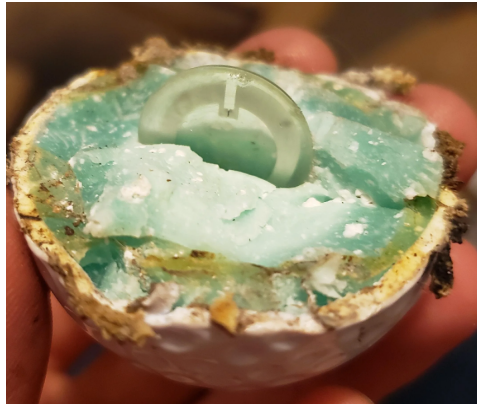
Figure 3.21 RFID Tag Embedded in Golf Ball (Awaiting Permission from Ok-Chemistry-2194)
