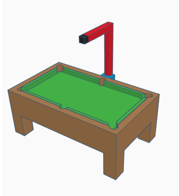
Figure 5.2: Example of Fixture Mounted Camera
