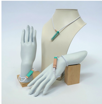
Figure 3.17: Maptic Haptic Feedback Apparatus (“Maptic is a wearable navigation system for visually impaired people”) (Awaiting Permission from Dezeen)
