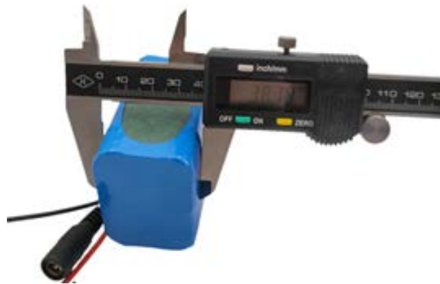
Figure 25 - 18650 Battery Pack Dimensions
