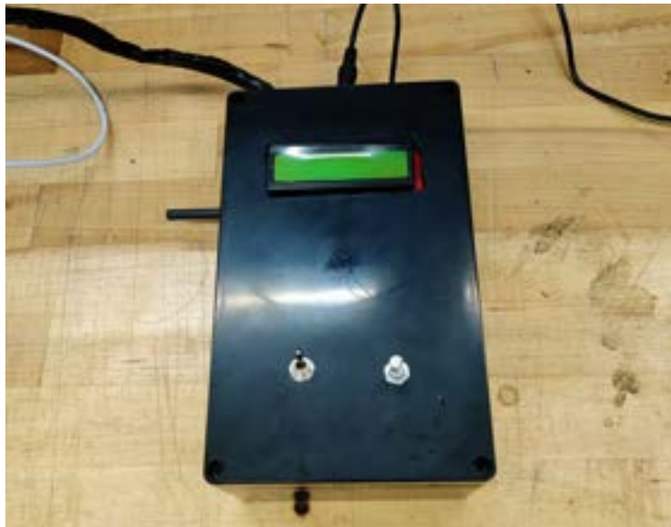
Figure 12 - Picture of control box / housing from completed project
