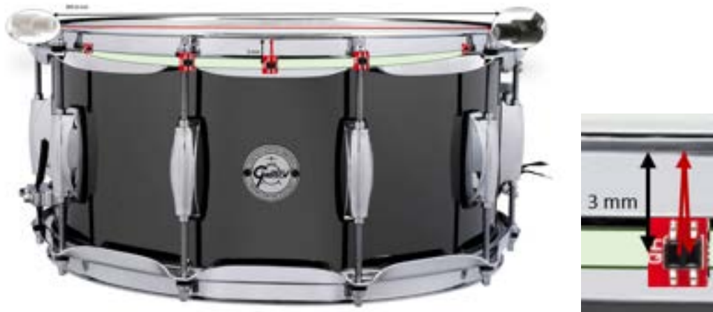
Figure 20 - Diagram of the LUDS's optical design (left) and close up of a reflectance sensor (right)
