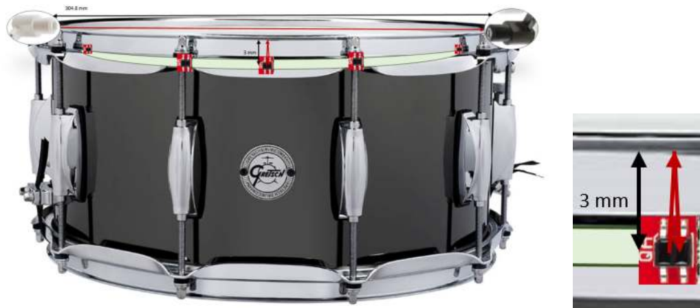
Figure 21 - Diagram of the LUDS's optical design (left) and close up of a reflectance sensor (right)
