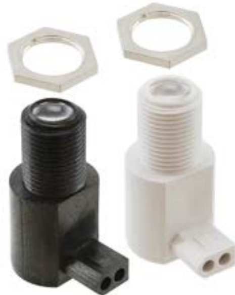
Fig. 4. OPB856Z’s show with their special housing.
