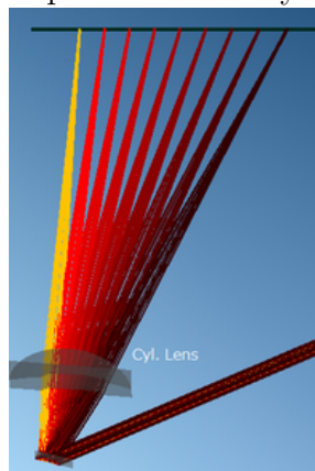
Figure 56: Spectrometer Ray illustration
