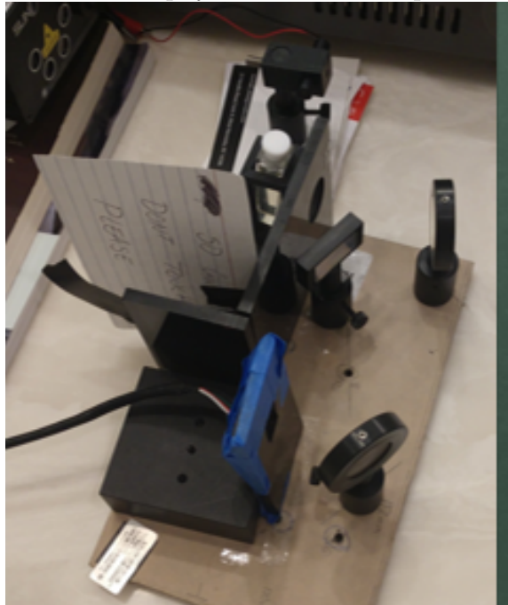
Figure 4: Chlorophyll Fluorescence Spectrometer
