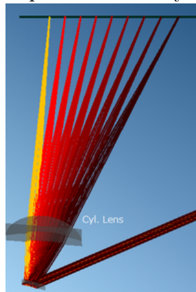
Figure 59: Spectrometer Ray illustration
