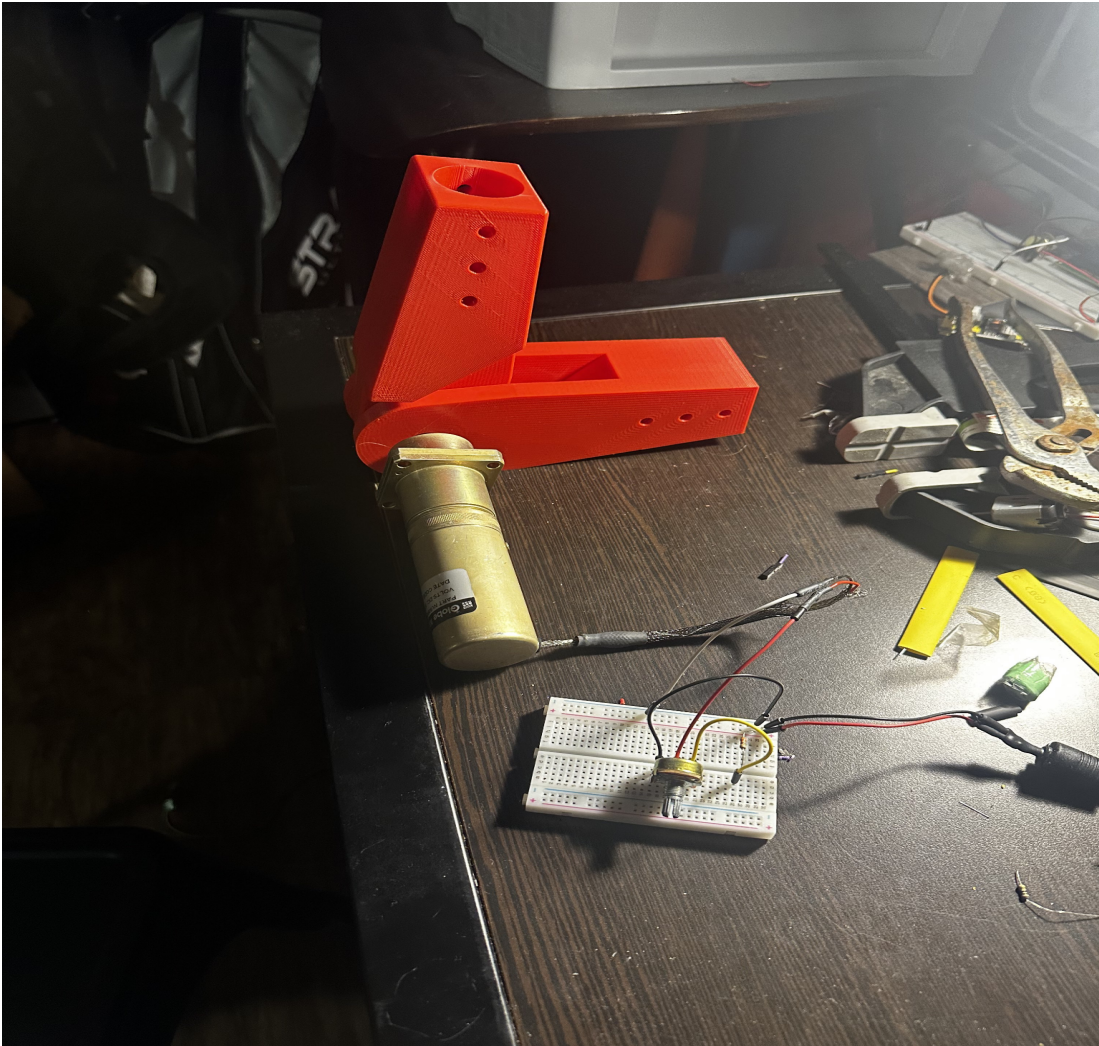
Figure 3.9.2 DC Brushed Motor Test with 3D Printed Joint
