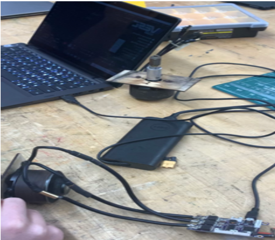
Figure 3.9.3 DC Brushless Motor Test with Software
