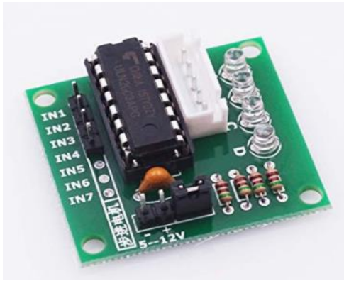
Figure 10, UL2003 Driver Board (left), L298N Motor Driver Control Board (right)
