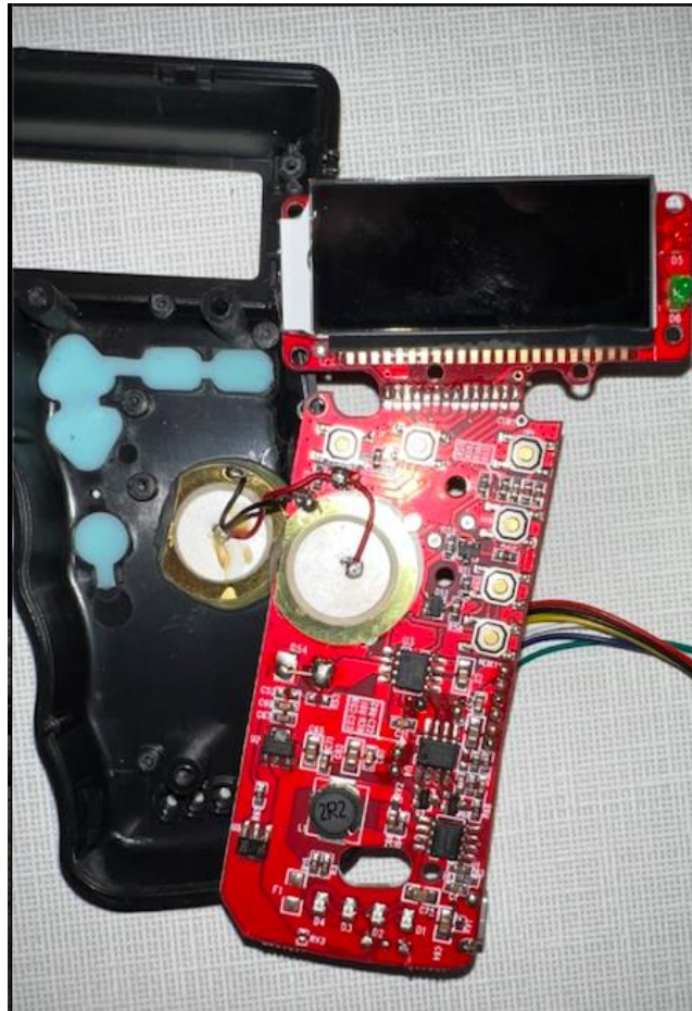
Figure 36, Jowoom Automatic Tuner (deconstructed) showing two piezoelectric sensors in parallel
