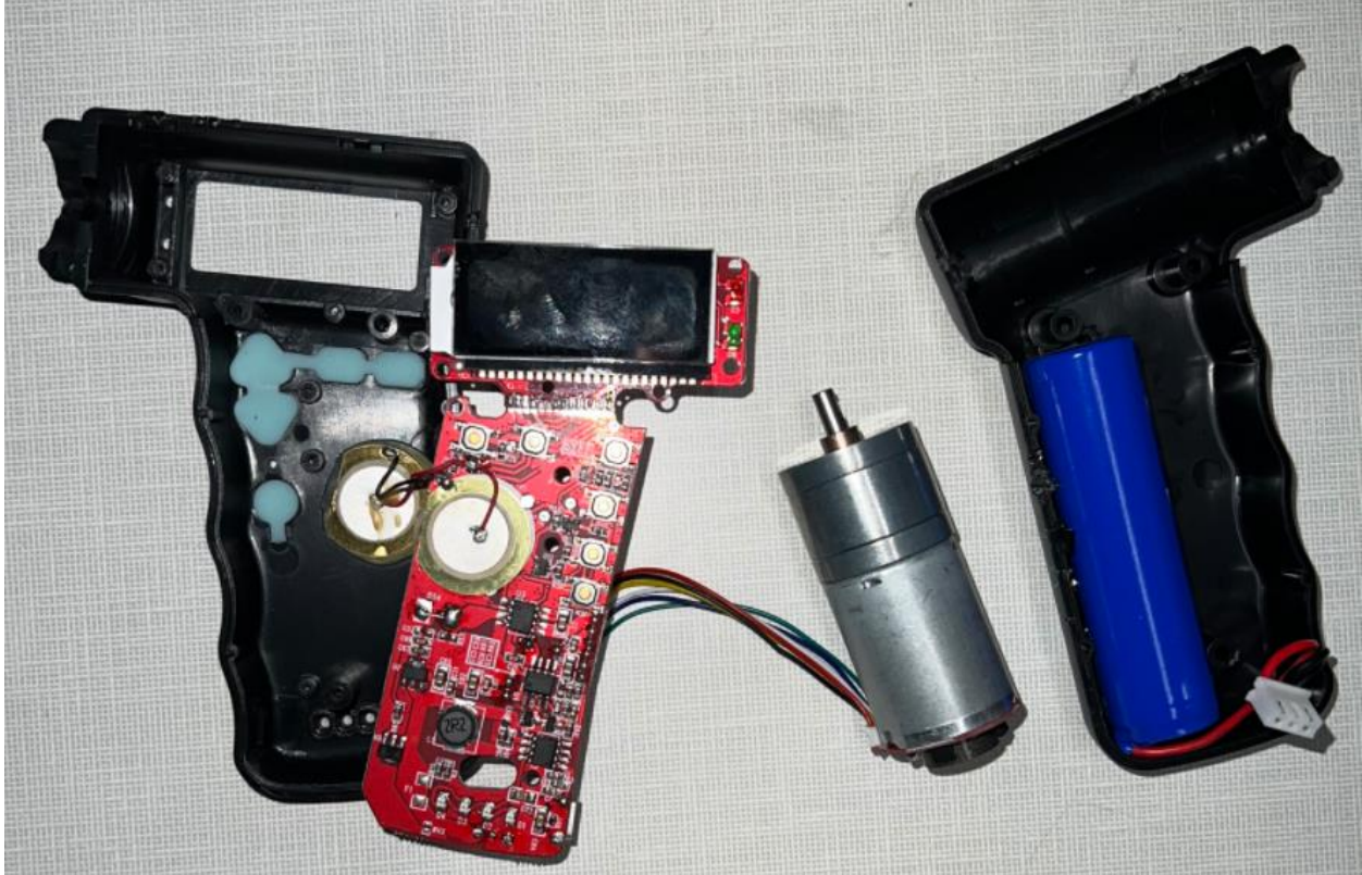
Figure 31, Jowoom internals front side
