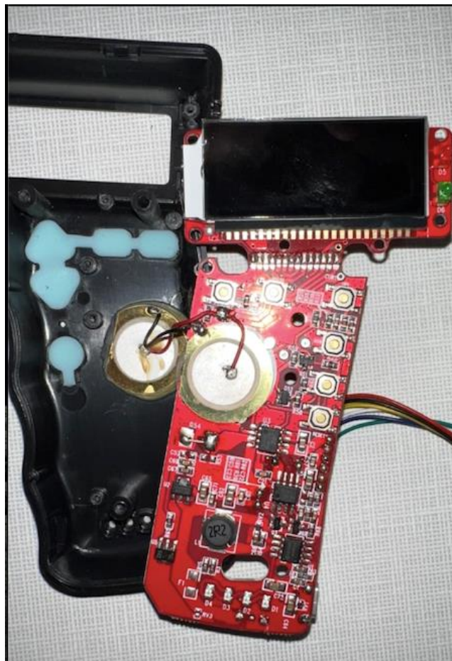
Figure 33, Jowoom Automatic Tuner (deconstructed) showing two piezoelectric sensors in parallel
