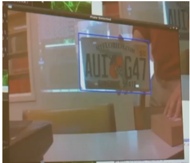
Fig 7. OpenALPR identifying license plates and extracting information
