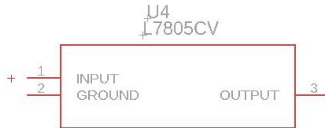
Figure 20: LM-7805 Integrated Circuit diagram
