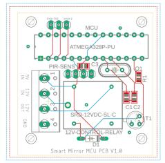
The PCB was manufactured in Hong Kong and then assembled by the team. The image below shows the final product. A 28-pin dual inline package was used in place of soldiering in the MCU to the board. This decision was made to make boot loading the chip easier, as well as make future programming changes as easy as possible.
