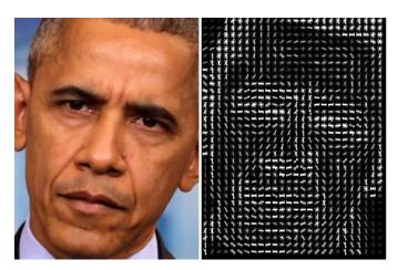
When a user stands in front of the smart mirror, the camera will take a photo, and run the algorithm within a few seconds to determine if a known user is present. The vanity lights that are included in the mirror are helpful in this process, because for best results, a user wants to be in a well lit area. However, HOG is an algorithm known to work well from
