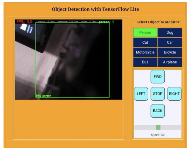
Fig. 10. Webapp portrayal of object detection using TensorFlow
