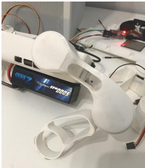
Fig. 1. Image showing example of leg mounted onto the lower body of the robot.
