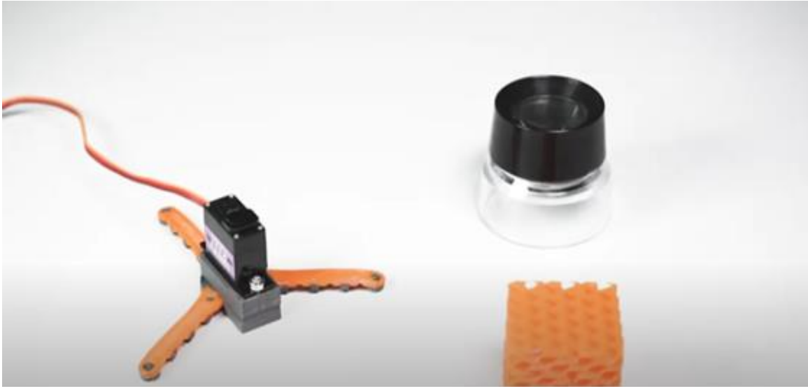
Figure 32: Flexible gripper at rest (Courtesy Layershift)
