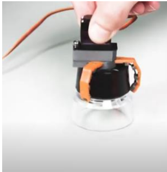
Figure 33: Flexible Gripper Actuating (Courtesy Layershift)
