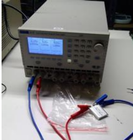
Figure 11: Battery Charging from a DC Power Supply
