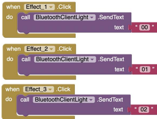
Fig. 6. Block programming for ICT effects.
