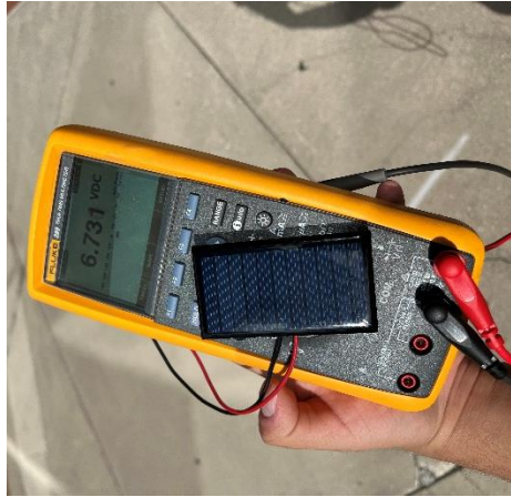
Figure 23 - Solar Panel voltage testing
