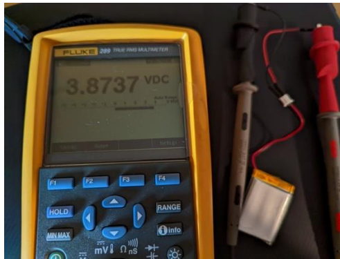
Figure 22 - Battery Open-Circuit Voltage
