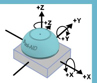
MPU-6050 Orientation & Polarity of Rotation
