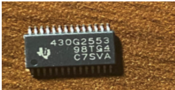
Fig.3. Picture of the MSP430G2553 used to control the servomotors
