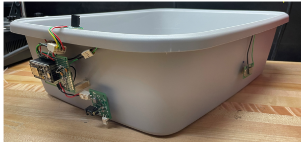
Figure 57: Completed waste station.
