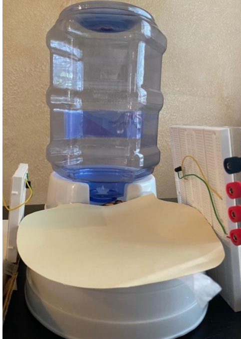
Figure 70 IR LED and Photodiode Setup
