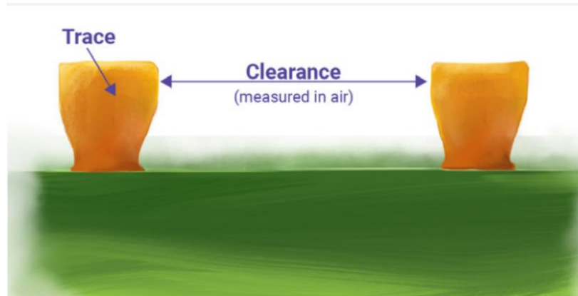
Figure 74 Example of clearance between traces on PCB
