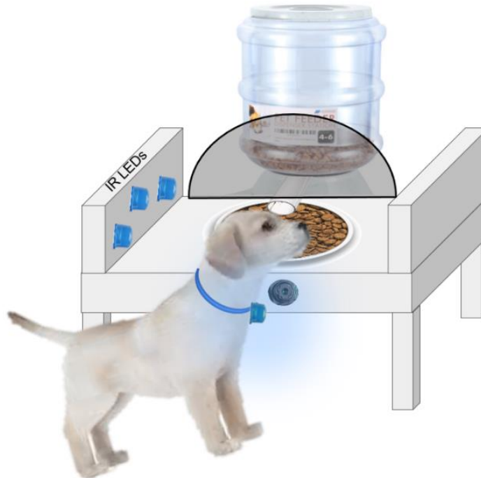
Figure 46 Opto-Smart Pet Bowl IR LED Layout
