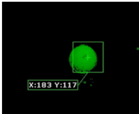
Figure 3-5 Example of color object tracking (Courtesy of roborealm.com)
