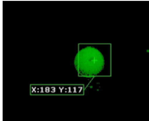
Figure 11 Example of color object tracking (Courtesy of roborealm.com)
