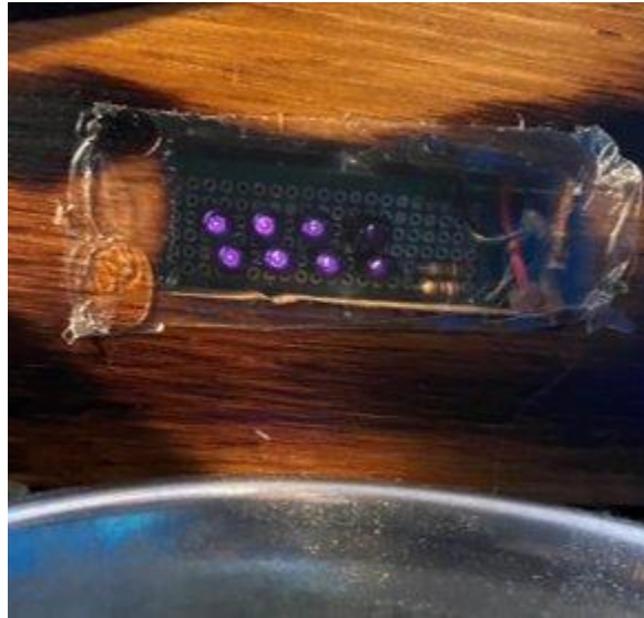
Figure 49 Opto-Smart Pet Bowl IR LED Layout
