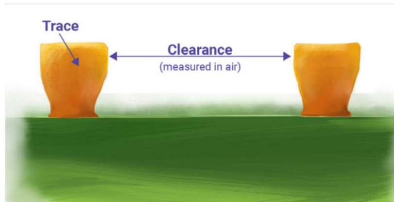
Figure 85 Example of clearance between traces on PCB
