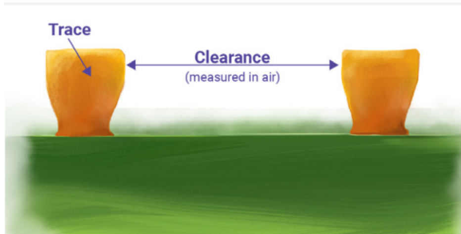
Figure 37 Example of clearance between traces on PCB
