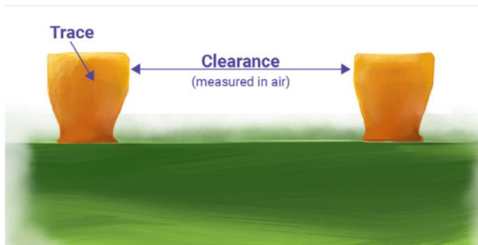
Figure 65 Example of clearance between traces on PCB
