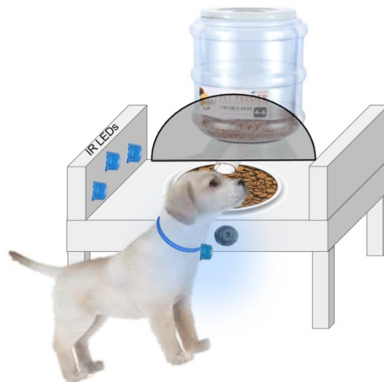
Figure 49 Opto-Smart Pet Bowl IR LED Layout
