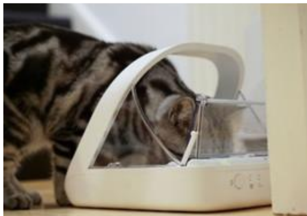
Figure 7 Existing Automatic Feeder Design with Self-Opening/Closing Lid
