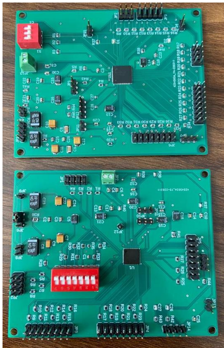
Figure 13. Assembled Serializer & De-Serializer PCB
