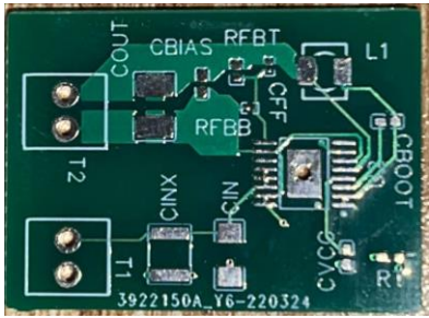
Figure 10. Unassembled Power Supply PCB
