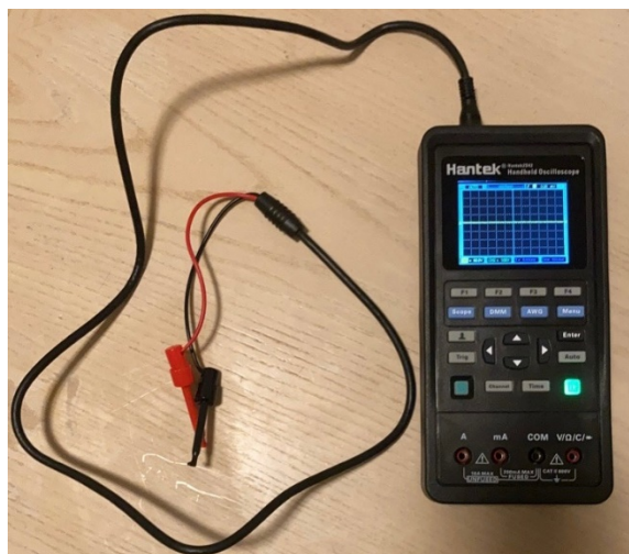
Figure 80: Hantek 2D42 3-in-1 Oscilloscope used to read photodiode output
