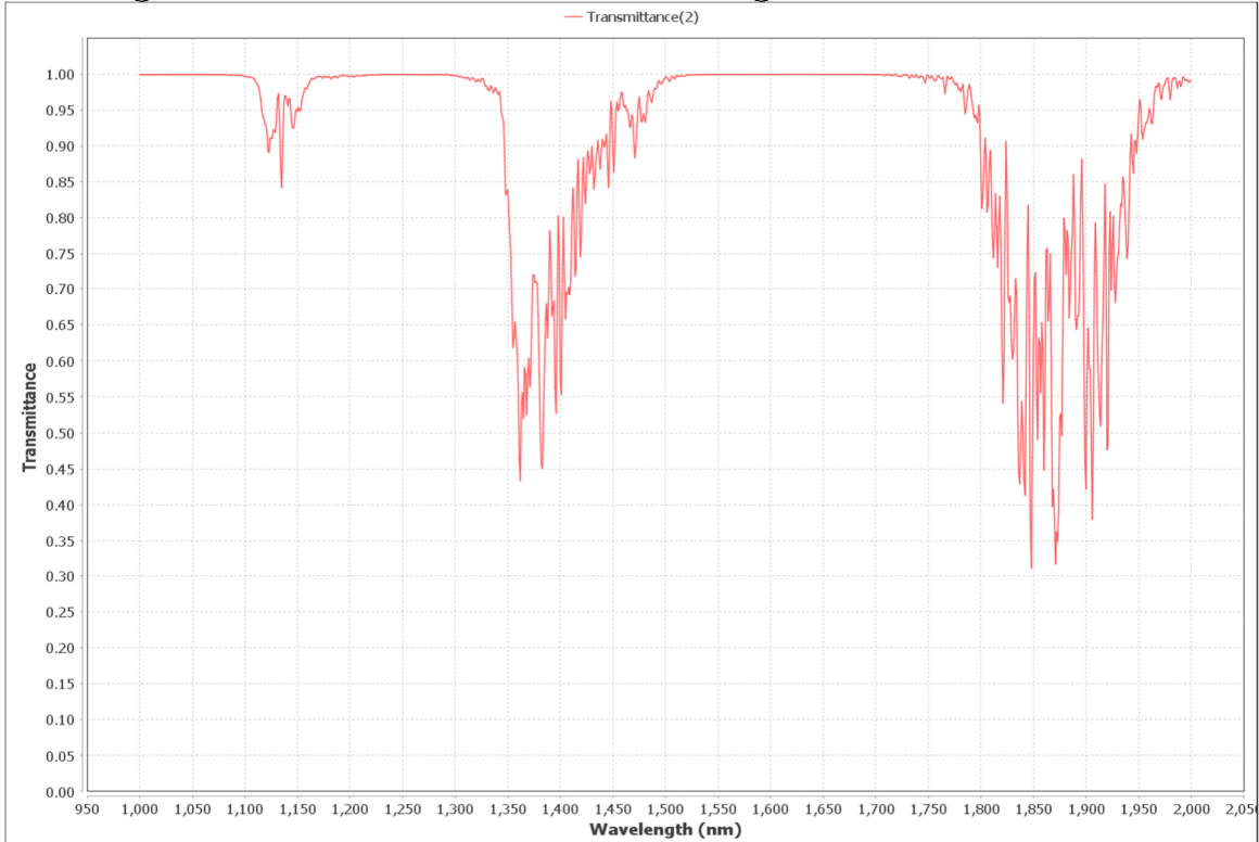
Figure 58: Transmittance over a 1km range as a function of wavelength for a Mid-Latitude Summer Atmosphere as modeled in MODTRAN
