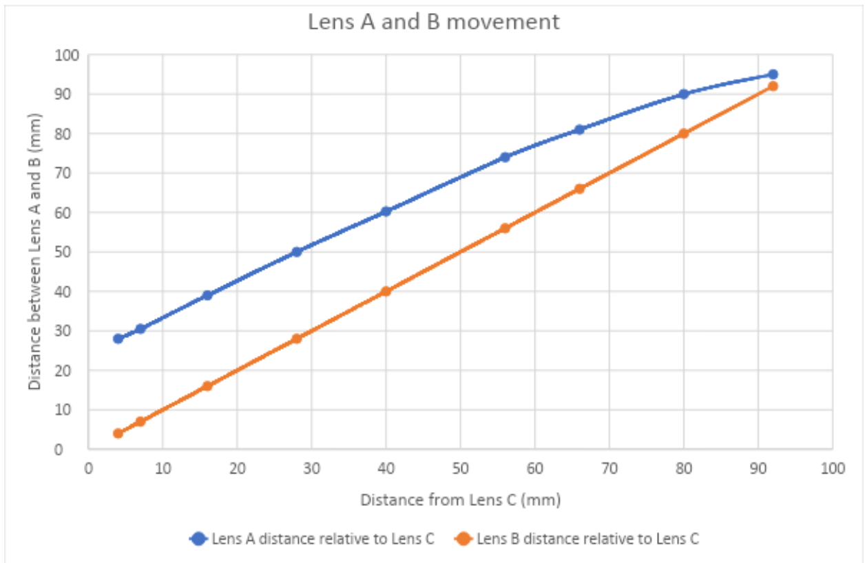
Figure 24: Graph depicting the movement of compensator lens A, and variator lens B, relative to stationary prime lens C. Imagine lens C laying along the x axis, and each point representing a different location along the optical axis. The trend line represents the movement of the lens being linear in the case of the variator lens and nonlinear in the case of the compensator lens.
