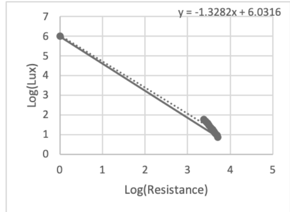
Figure 12. Log(Lux) Vs Log(Resistance) of 5506 LDR. The slope equation is used for calibration of the Lux Meter.
